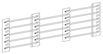
Remember that with a 4 bracket configuration the load weight will increase proportionally so ensure that the wall is capable of taking the load.
